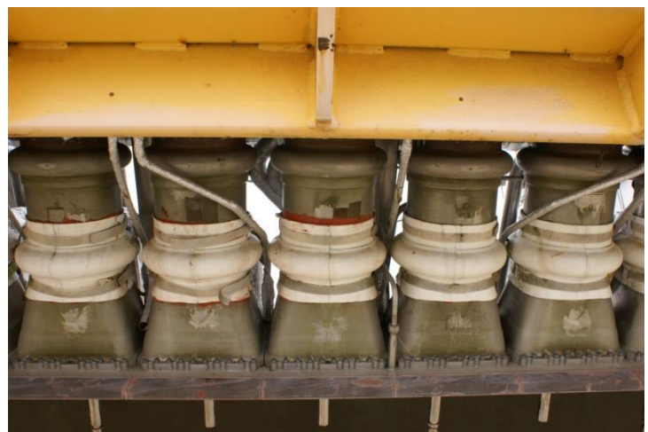
FIGURE 15: RS-2200 engine (without turbopump) in shipping crate Figure 16: five of twenty 9.3" diameter thrusters
