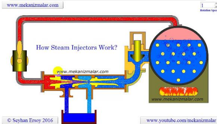
FIGURE 18: Steam Injector animation (with control valve on left and one-way valve before boiler)
