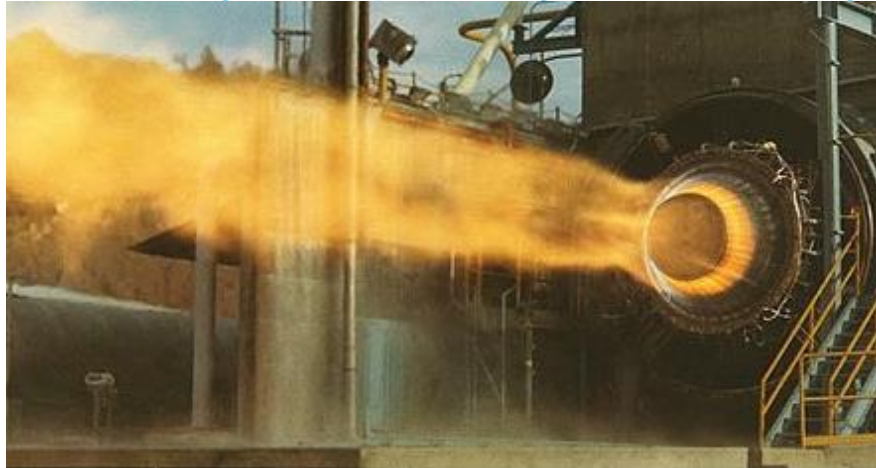
Figure 14: 250k lb Toroidal Aerospike engine, based upon the J-2 engine from the 2 nd & 3 rd Stage of the Saturn V.
